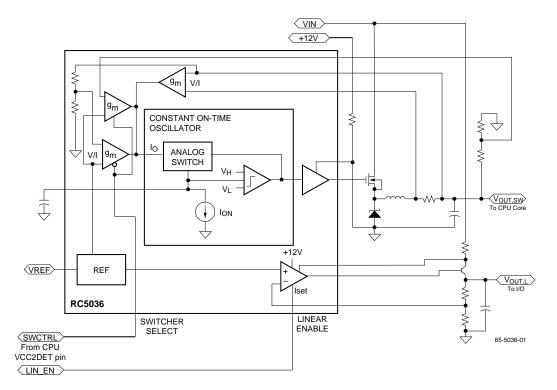
Figure 3. RC5036 Block Diagram
