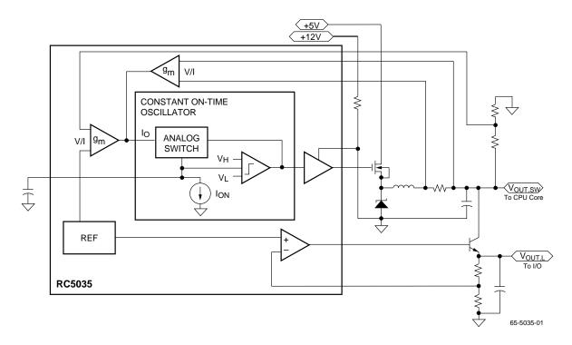
Figure 4. RC5035 Block Diagram
