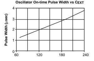
Figure 12. Pulse Width vs. Capacitance
