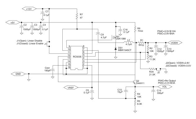
Figure 7. RC5035 Implementation for P54/P55C/K6 Flexible Motherboard
