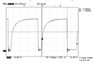
Figure 10. Scope Photo of Pin 9 at a 5Amp Load
