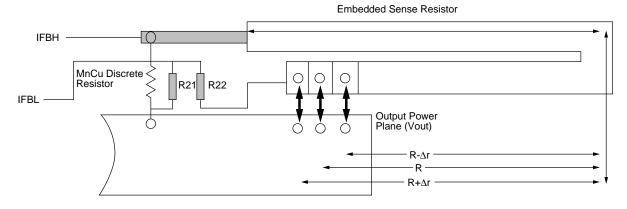
Figure 16. RC5036 Demo Board Sense Resistor Implementations
