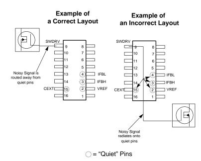
Figure 13. Example of Correct and Incorrect Layout
