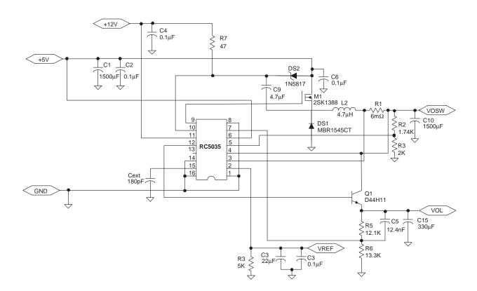
Figure 6. RC5035 with Linear Regulator Slave
