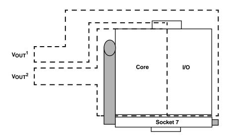
Figure 1. Dual Power Plane with Socket 7 for P55C
