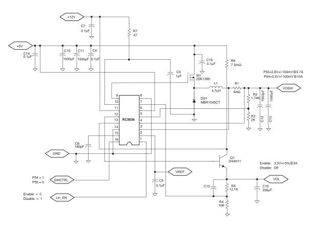
Figure 5. Dual Power Supply for P54/P55C/K6 Flexible Motherboard
